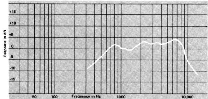
Frequency response contour of Model 2470 coupled to a 2350 horn. Measured response of a typical production unit, including all peaks and dips, does not deviate more than 2 dB from the above curve.
